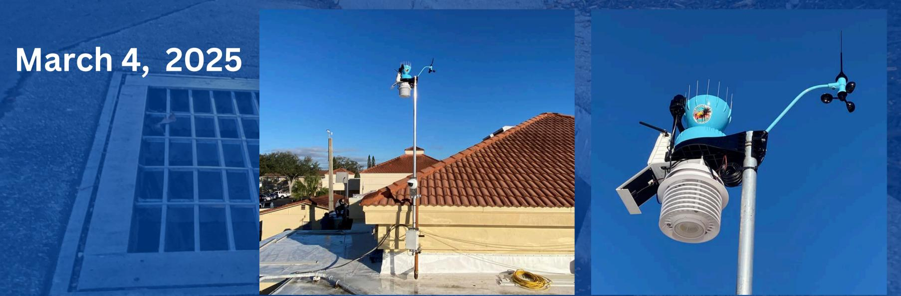
The City has installed a weather station atop City Hall that measures atmospheric conditions which will be used to document our stormwater system's performance compared to measured rain events.
